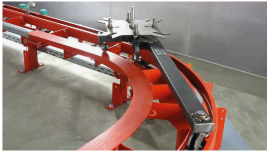
E-Conveyor iP&F with individually designed outrigger.
